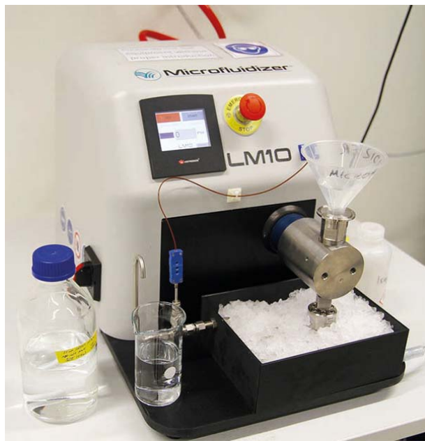
The LM10 microfluidizer from Microfluidics presses a cell suspension through a shearing cell, a ceramic unit, which becomes increasingly narrow and destroys the cell at a given moment. Then the lysate, with the proteins in it, goes through a part that cools very efficiently.
