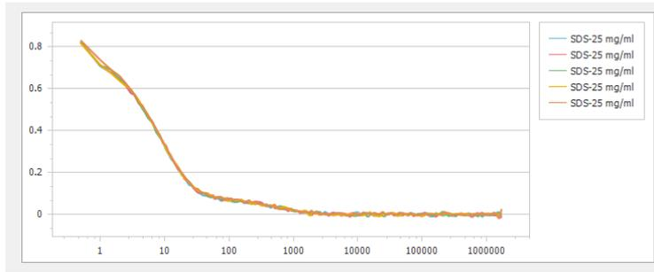
Figure 4. The overlap of correlation function of 25mg/mL SDS self-assembled micelle
