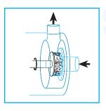
The high shear action of the rotor/stator workhead progressively reduces the size of the polymer particles, exposing an increasing surface area of polymer to the surrounding asphalt.
