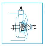
Asphalt and polymer are drawn into the workhead of the In-Line mixer. High speed rotation exerts hydraulic shear on the materials.
