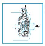
The asphalt and polymer mixture is forced out through the stator and recirculated back into the vessel by the self-pumping action of the In-Line mixer. The combination of finely reduced particle size and vigorous mixing rapidly solubilizes the polymer.
