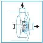
Centrifugal force drives the materials to the periphery of the workhead where they are reduced to a fine droplet/ particle size in the gap between the rotor blades and the inner wall of the stator.
