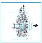
Further reduction in particle size follows as the mixture is forced out through the stator, increasing the surface area of reagent exposed to the oil. This accelerates the reaction, and maximizes the yield.
