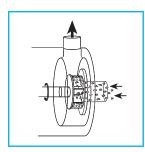
Stage | The slurry is drawn into the rotor/stator workhead and is driven to the periphery of the head by centrifugal force.
