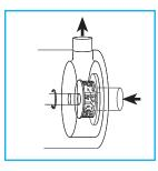
Stage 2 Agglomerates are subjected to a milling action in the clearance between the tips of the rotor blades and the inner wall of the stator
