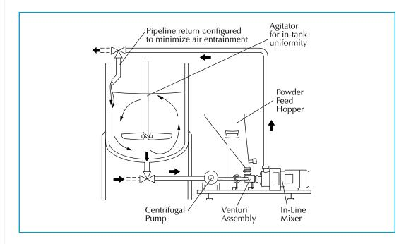
The base liquid is drawn from the vessel by the centrifugal pump and passed through the venturi assembly into the In-Line Mixer. The high velocity flow through the venturi creates a vacuum in the chamber below the powder hopper. The liquid is returned to the vessel by the self-pumping In-Line Mixer.
