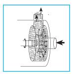
Further reduction in particle size follows as the mixture is forced out through the stator, increasing the surface area of reagent exposed to the oil. This accelerates the reaction, and maximizes the yield.
