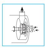
The reagent is introduced to the oil just prior to the intake of the Silverson mixer. The ingredients are drawn into the rotor/stator workhead and vigorously mixed
