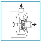
Centrifugal force drives the materials to the periphery of the workhead where they are reduced to a fine droplet/ particle size in the gap between the rotor blades and the inner wall of the stator.
