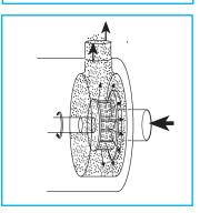
The product is forced out of the stator as fresh material is drawn into the workhead. A circulatory mixing cycle develops in which all the material passes through the Silverson workhead.
