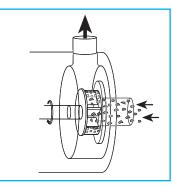
The high speed rotation of the rotor blades creates a powerful suction which draws the liquid and solid/powdered ingredients into the workhead.
