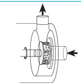
The materials are subjected to intense shear in the confined area of the workhead. Agglomerates are broken down in the gap between the rotor blades and stator wall. A lump-free mixture is rapidly obtained.
