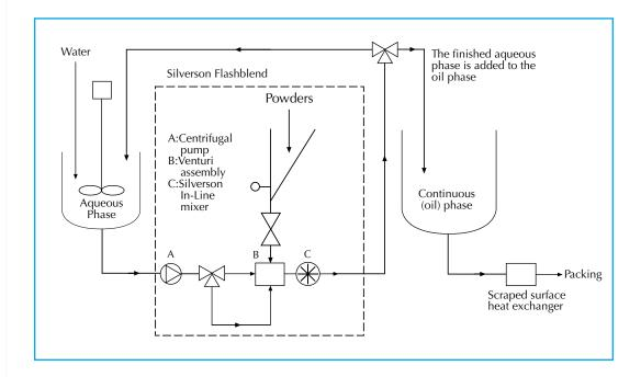
Water is drawn from the vessel into the Flashblend by the centrifugal pump (A) and forced through the venturi assembly (B) into the In-Line Mixer (C). The high velocity flow through the venturi creates a vacuum in the chamber below the powder hopper. Powders can be fed into the hopper without the need for premixing.
