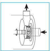
The materials are subjected to intense shear in the confined area of the workhead. Agglomerates are broken down by the intense mixing action. A lump-free mixture is rapidly obtained
