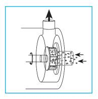
The high speed rotation of the rotor blades creates a powerful suction which draws the liquid and solid/powdered ingredients into the workhead. These can be added without the need for pre-mixing
