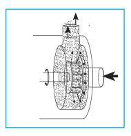
The product is forced out of the stator as fresh material is drawn into the workhead. A circulatory mixing cycle develops in which all the material passes through the Silverson workhead. The oil phase ingredients are added to the vessel and emulsified into the water.
