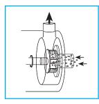
The vessel is charged with liquid and the mixer is started. The powdered ingredients are added without prior heating of the liquid. The high speed rotation of the rotor blades creates a powerful suction which draws liquid and solid ingredients into the workhead and rapidly mixes them.
