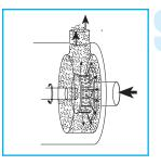
As the product is forced out through the stator, fresh powdered and liquid ingredients are drawn into the workhead and processed as before. A circulatory mixing pattern is set up within the vessel, ensuring all material is passed through the workhead many hundreds of times. A stable suspension of active ingredients is rapidly achieved
