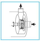
The sugar granules are reduced in the gap between the rotors and stator wall. Increasing areas of powdered and solid ingredients are exposed to the surrounding liquid and dissolved. The active ingredients are similarly reduced to a low particle size and fully coated by the surrounding liquid. This creates a very fine and stable suspension.
