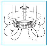
Once the powdered ingredients have been fully dispersed in the "continuous" liquid phase, the "dispersed" phase is added. The high shear mixing action of the workhead forms a uniform and stable emulsion.
