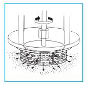
The solids are de-agglomerated in the precision machined workhead before being forced out through the stator and circulated back into the mix. Simultaneously fresh material is drawn into the workhead.
