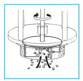
The vessel is charged with appropriate base fluid. The mixer is started, and the solid/ powdered ingredients are added. The powerful suction created by the high speed rotation of the rotor draws liquid and solids into the workhead where they are rapidly mixed.
