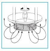
The continuous intake and expulsion of materials through the workhead progressively reduces particle size and exposes an increasing surface area to the solvent, accelerating the solubilization process. Premicronized pigments and other powdered or liquid ingredients can be added and are dispersed/ deagglomerated as they are subjected to intense high shear with each pass through the workhead.
