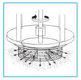
The resin chips are subjected to a milling action in the gap between the tips of the rotor and the inner wall of the stator, rapidly reducing particle size. The product is then forced out through the stator at great velocity as fresh material is drawn in.
