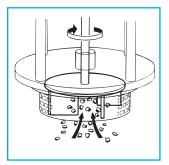
The vessel is charged with solvent and the resin chips are added. The high speed rotation of the rotor draws the liquid and solids up from the base of the vessel into the workhead. Centrifugal force then drives the materials to the periphery of the workhead.
