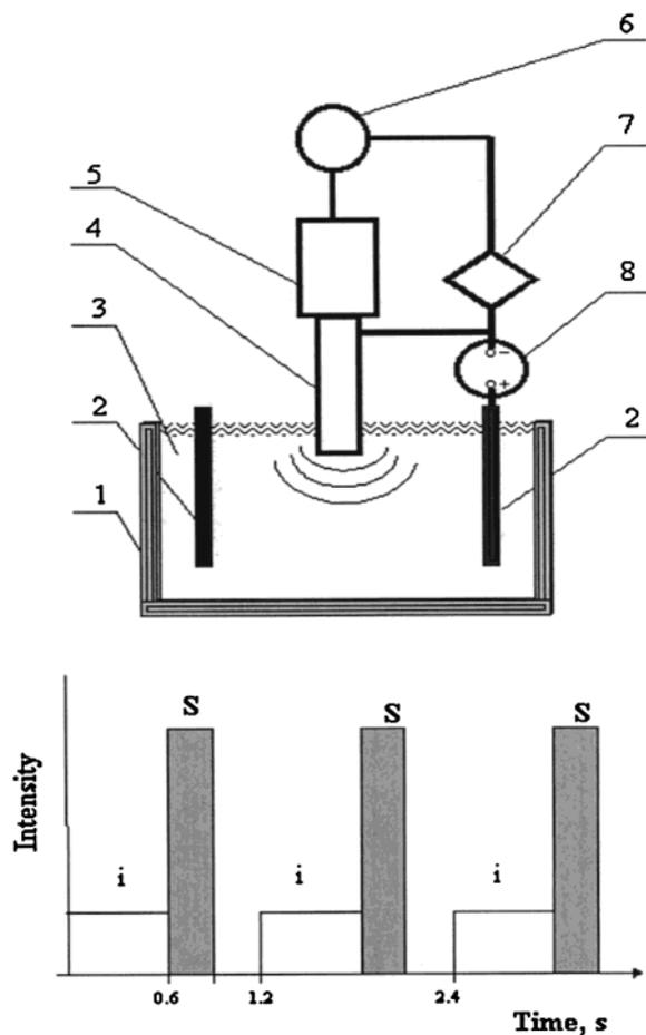
**Figure 1.** Experimental setup and sonoelectric cycle. Top: 1, vessel; 2, anode; 3, electrolyte; 4, sonic horn/cathode; 5, sonic driver; 6, sonicator's controller; 7, synchronizer; 8, dc power source. Bottom: i, electric current pulse of 0.6 s duration; s, sonic pulse of 0.3 s duration; the total cycle is 1.2 s long. The usual value of electric current density was 50 mA/cm<sup>2</sup>.
