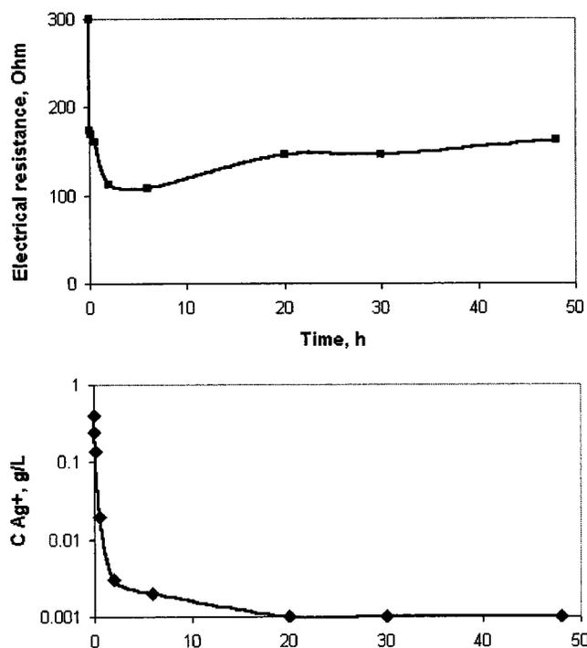
**Figure 4.** Electrical resistance and residual concentration of silver ions in the course of the sonoelectrochemical treatment. One can readily see that the system has reasonable conductivity while even completely depleted of silver ions.
