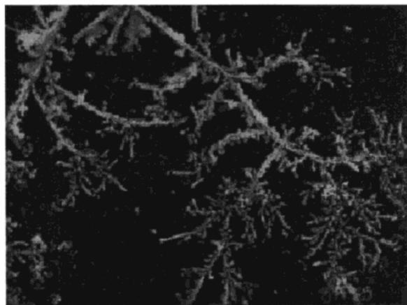
**Figure 6.** TEM picture of fractal-like agglomerate. Such shapes were obtained at low values (15 mA/cm<sup>2</sup>) of electric current.
