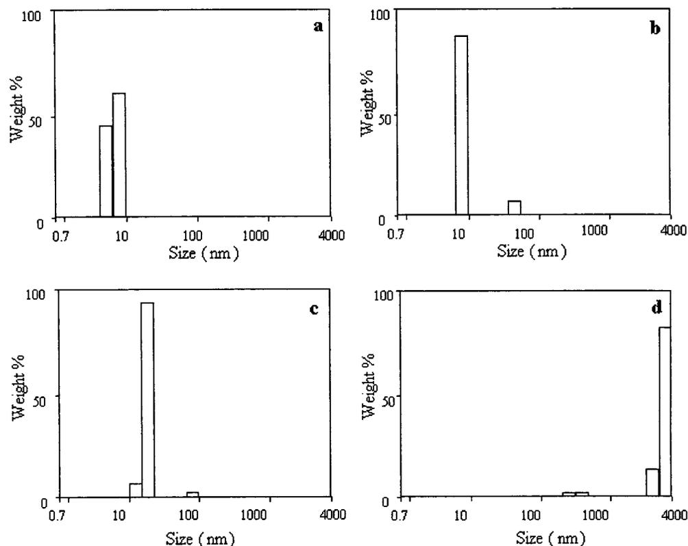
**Figure 3.** Particle size distributions as measured by the method of photon correlation spectroscopy: (a) 5 min, mean size 7.9 nm; (b) 25 min, mean size 11.4 nm; (c) 1 h, mean size 22.3 nm; (d) 56 h, mean size  $2.67 \times 10^3$  nm.
